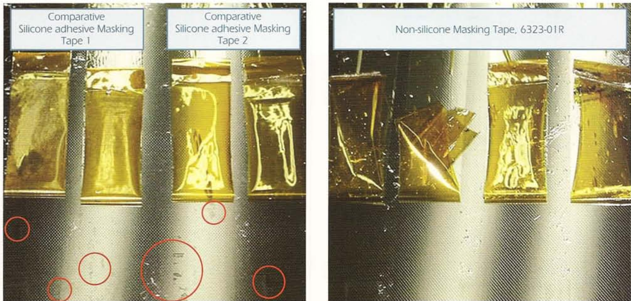
Low molecular weight polysiloxane contaminations observed in comparative silicone masking tape.
