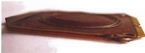
A double-sided circuit places copper on both sides of a dielectric layer.
