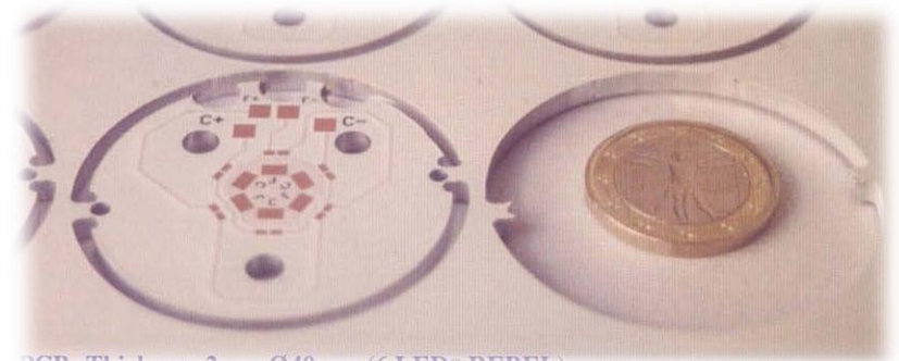
PCB: Thickness 2mm Ø40mm (6 LEDs REBEL)
